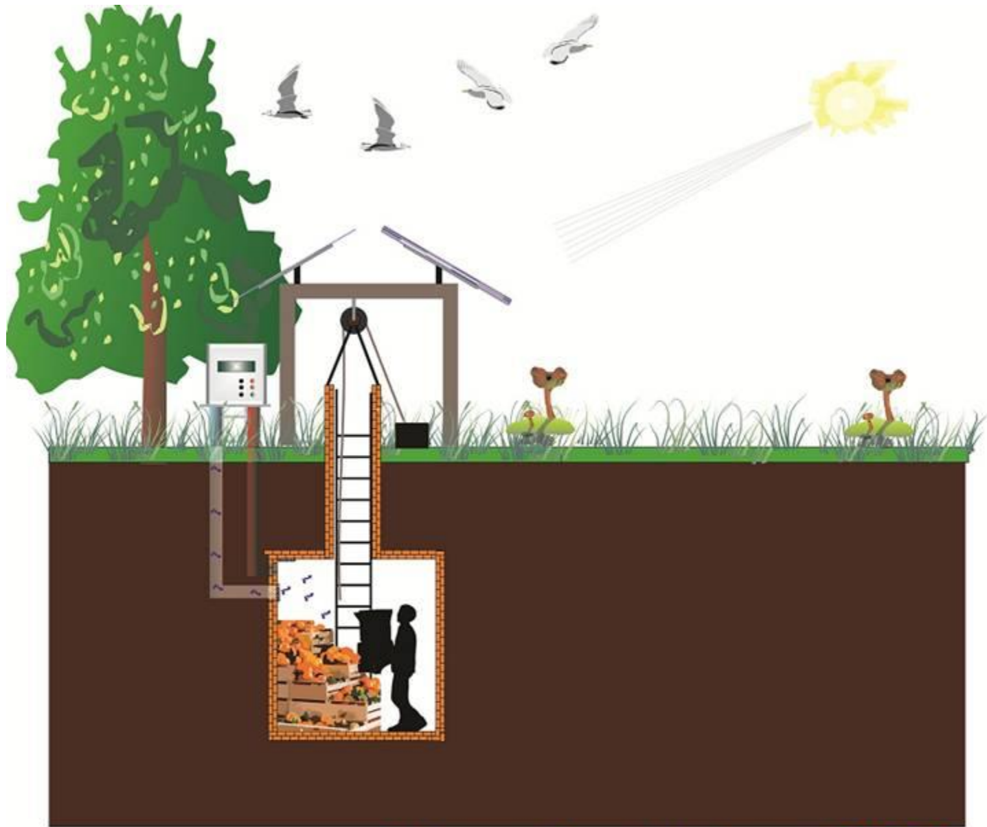
Solar earth cold storage (SECS)
